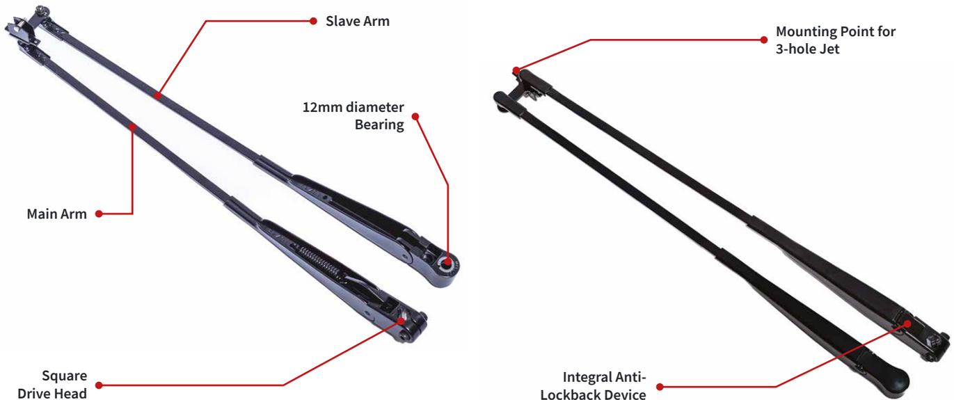
The wiper arms are finished in a semi-matt black colour process achieved by electro-phoretic paint deposition coupled with a further protective surface that prevents discolouration by ultra-violet light.
